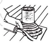
**Step 5:** Complete the flashing installation by fastening the metal flange down with fasteners at a spacing of  $1 \frac{1}{2}$ ".
