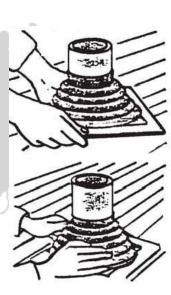
**Step 4:** Between the flashing base and the metal roof sheet apply silicone.
